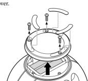
**2** Pull out the rechargeable battery upward, and
